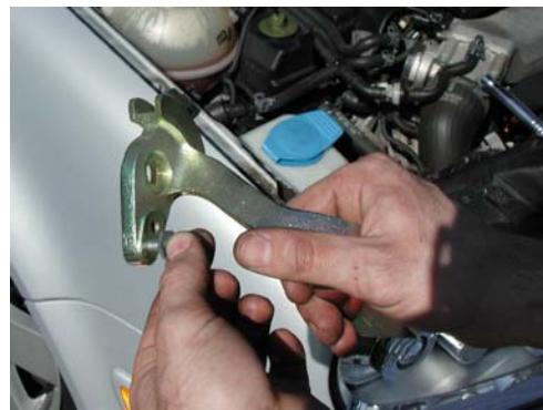
1. Screw the ball or pin into the desired position on the HPA Short Shifter and tighten with wrench. (20% position shown)
