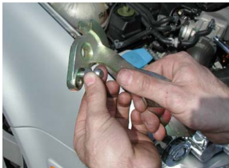
NOTE: Using the hole closest to the edge will give you a 20% reduction in shift throw. The hole closest to the spline will give you a 40% reduction on 02J models and 35% reduction on 02M models.
