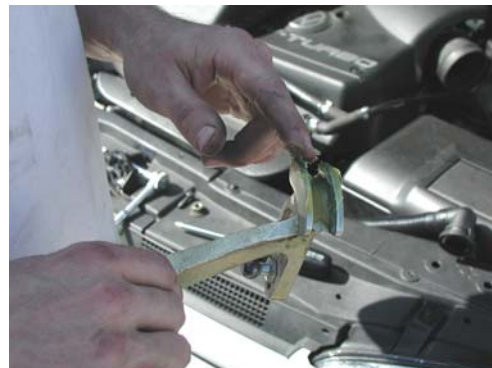
2. Put a bit of grease in the groove of the HPA Short Shifter.
