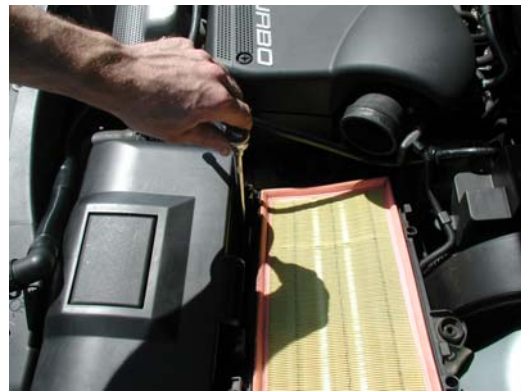
8. Remove bolt at front of lower airbox
