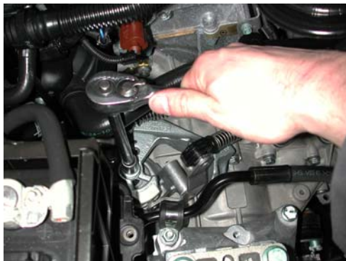
4. Re-install nut to hold shifter firmly in place. Tighten with 13mm socket.
