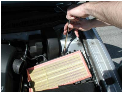
7. Remove bolt at back of lower airbox
