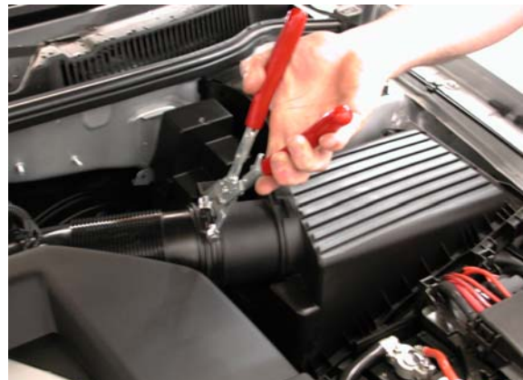
2. Using pliers or screwdriver, as needed, undo the clamp connecting the airbox.
