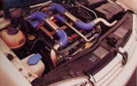
■ Nice symmetry accompanies the power. Twin turbos are seen up high, near the firewall.
