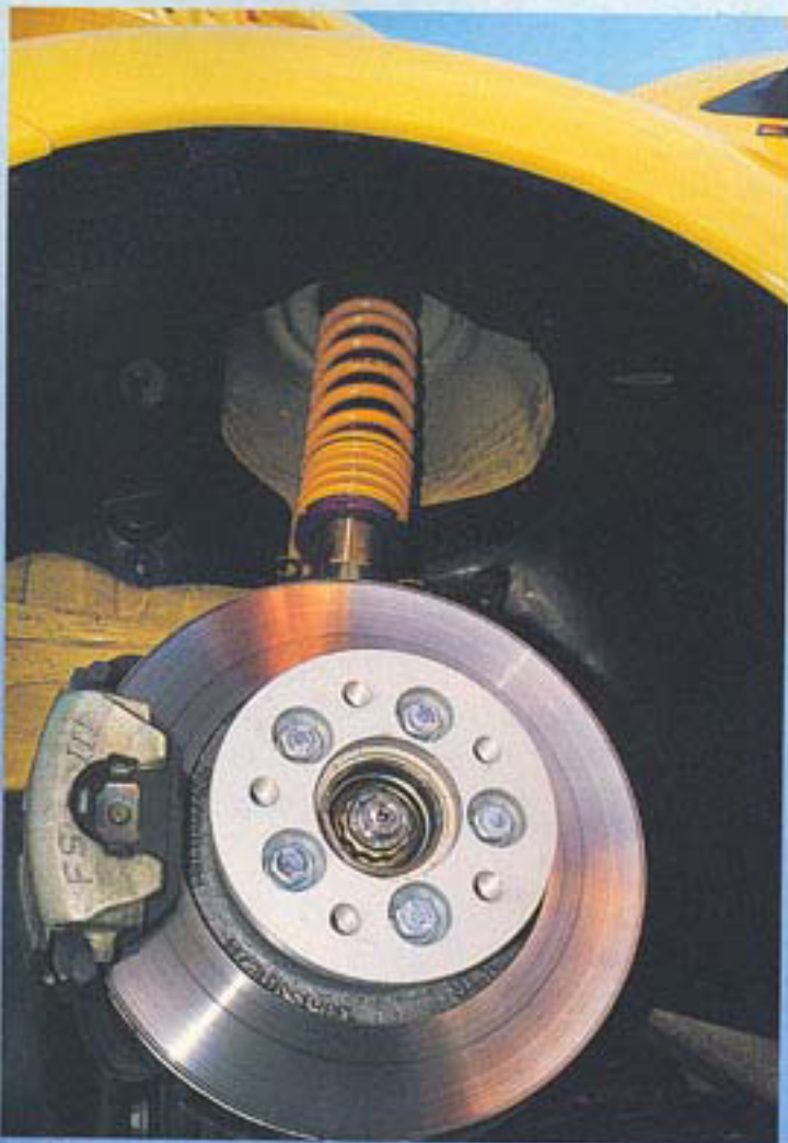
Gary's muscled Beetle uses KW fully adjustable coilover suspension, lowered 3" all round on the Bug's 8.5x17 wheels
