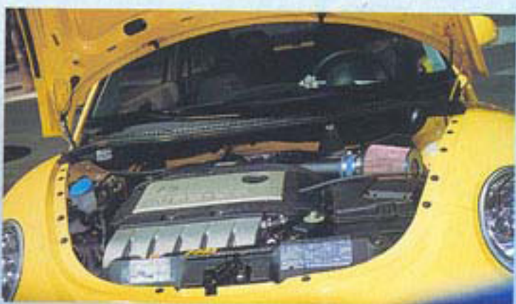
Mad grille (above left). Heart of the matter (below and above right) is a 2792cc, six cylinder, DOHC, fuel injected, 12v VR6
