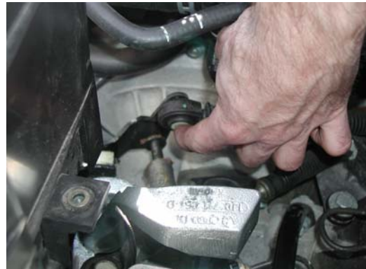
6. Push side-to-side linkage towards engine to disengage it from the shifter.
