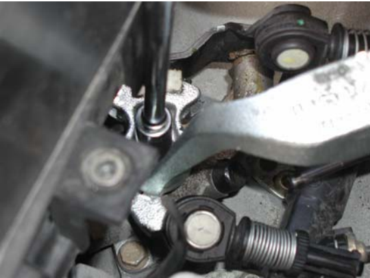
4. Using 13mm socket, remove the nut that is securing the shifter.
