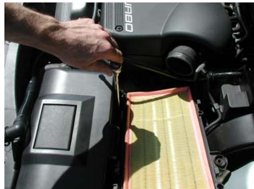
8. Remove bolt at front of lower airbox
