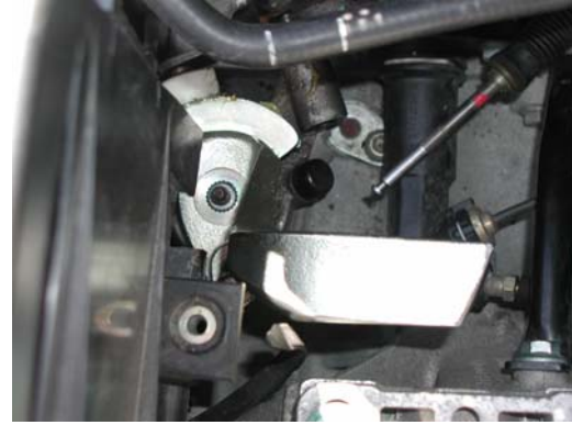
3. Carefully line up the index teeth of the splines and slide the HPA Short Shifter into place. This requires very little force if it is lined up properly.
