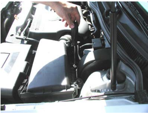
3. Loosen the two screws on back edge of upper airbox until threads are fully disengaged
