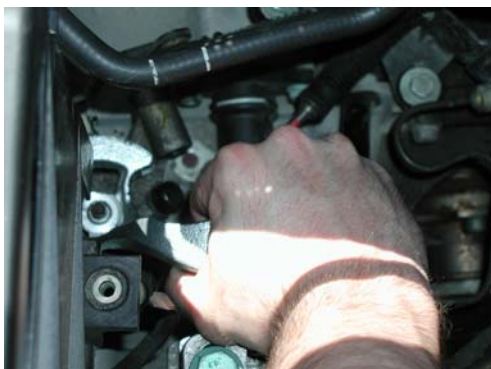
5. Slide the shifter off of the spline by grasping the counter weight of the shifter and wiggling it back and forth while pulling straight up.
