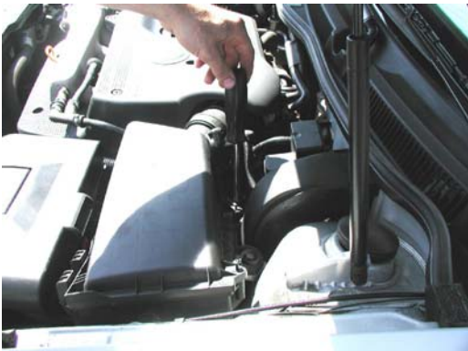
3. Loosen the two screws on back edge of upper airbox until threads are fully disengaged
