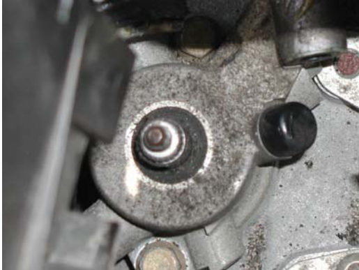
The index tooth on the male spline has a WIDE tooth.
