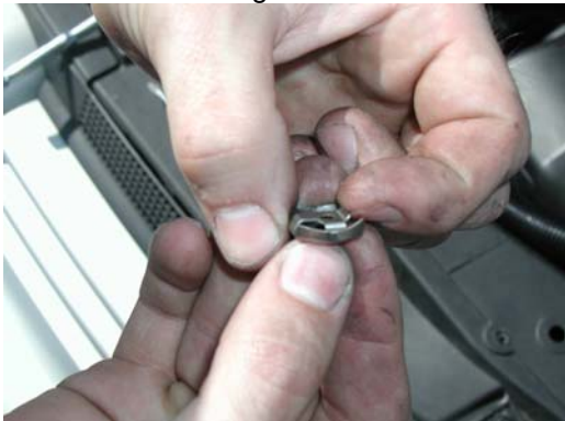
HINT: lift up on the locking lever in the center of the clip and then slide out.
