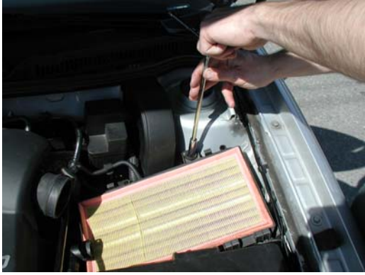
7. Remove bolt at back of lower airbox
