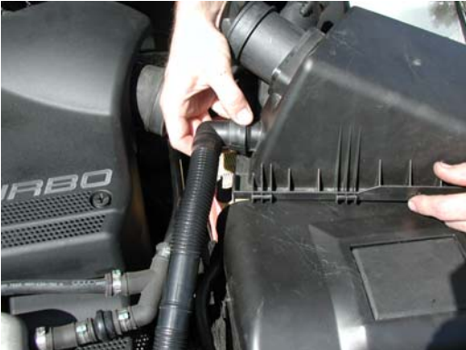
5. Disconnect air hose from engine side of upper air box - squeeze plastic retaining ring to disconnect (not applicable for all models.)
