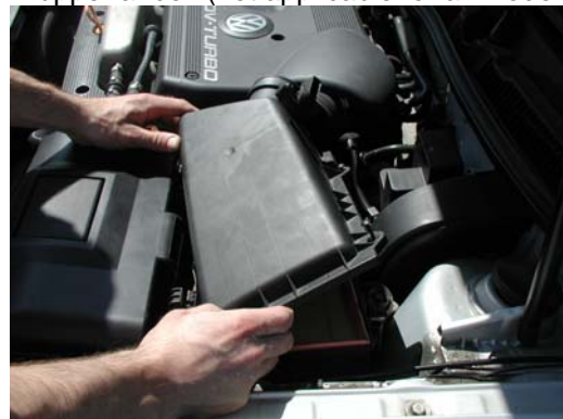
6. Slowly lift off upper air box and move out of the way
