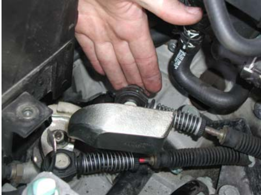
6. Slide the side-to-side linkage into place so it engages with the groove on the HPA Short Shifter
