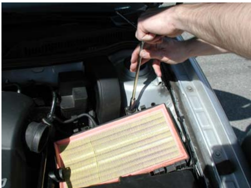
7. Remove bolt at back of lower airbox
