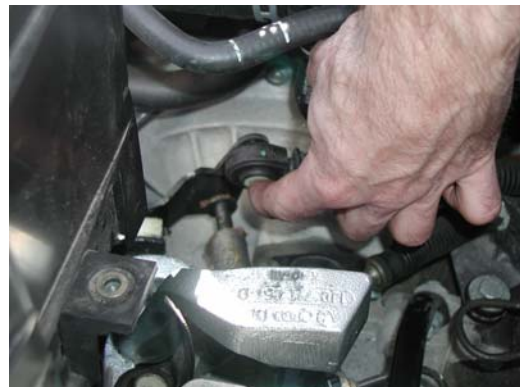
4. Push side-to-side linkage towards fender to disengage it from the shifter.
